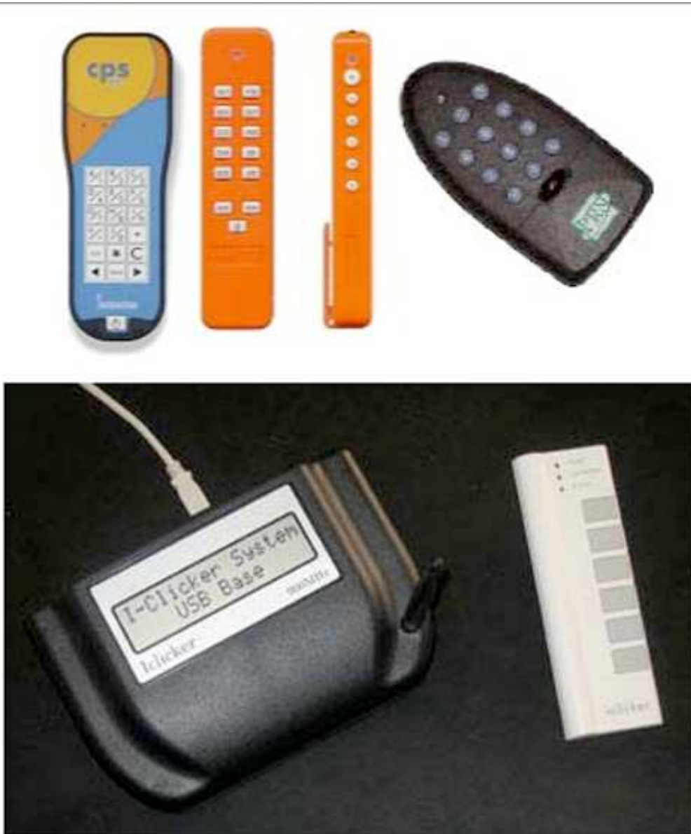
Figure 3. Infrared transmitters (top) and radio (RF) receiver and transmitter (bottom).
