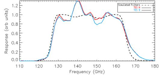
**FIGURE 2.** Measured Spectrum of a Prototype Pixel. Plotted are the simulated filter response function as well as the measured spectral response for polarization channels A and B. Note that the response for channels A and B were scaled so that the lower edge of the band roughly matched the simulated results.
