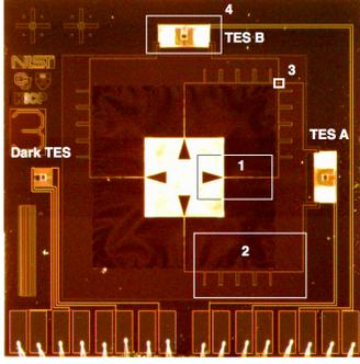
**FIGURE 1.** Photograph of prototype pixel. Boxed are: (1) Planar OMT fin to CPW-microstrip transition, (2) microstrip bandpass and lowpass filters, (3) microstrip crossover, and (4) TES island with TES and lossy-gold absorbers. Also labeled are the two polarization channels, A and B as well as the dark channel that is not connected to the OMT. The dark channel is used for diagnostic purposes.
