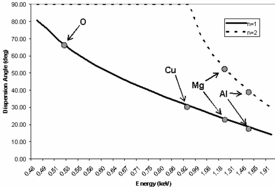
Figure 8: Predicted dispersion angles as a function of energy at first and second order. The energies of relevant lines are labeled. The graze angle on the monochromator grating is 0.75 degrees in this case.
