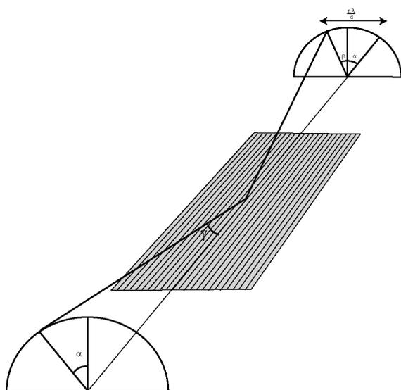
Figure. 1: Geometry of the off-plane mount. Quasi-parallel light at grazing incidence is diffracted in a cone around the direction of the rulings.
