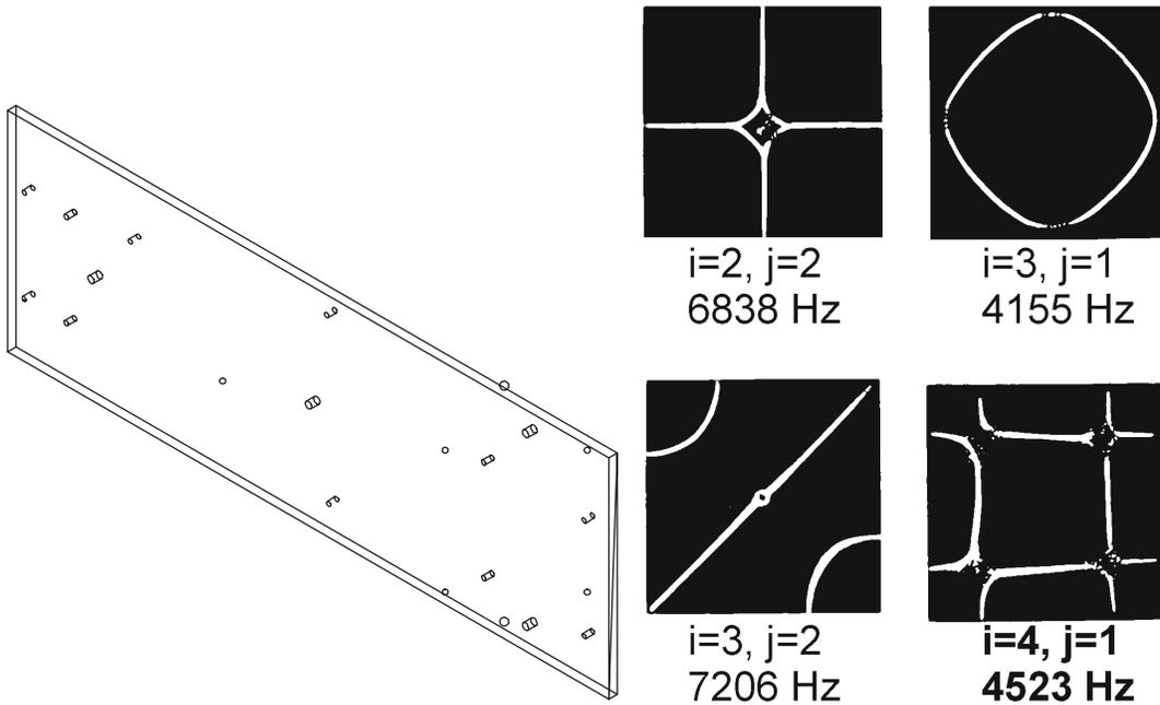
Figure 4: On the left is a CAD drawing of the base plate. On the right are possible vibration modes. The  $i=4, j=1$  mode on the lower right gives convenient node lines along which supports to the plate could be mounted.
