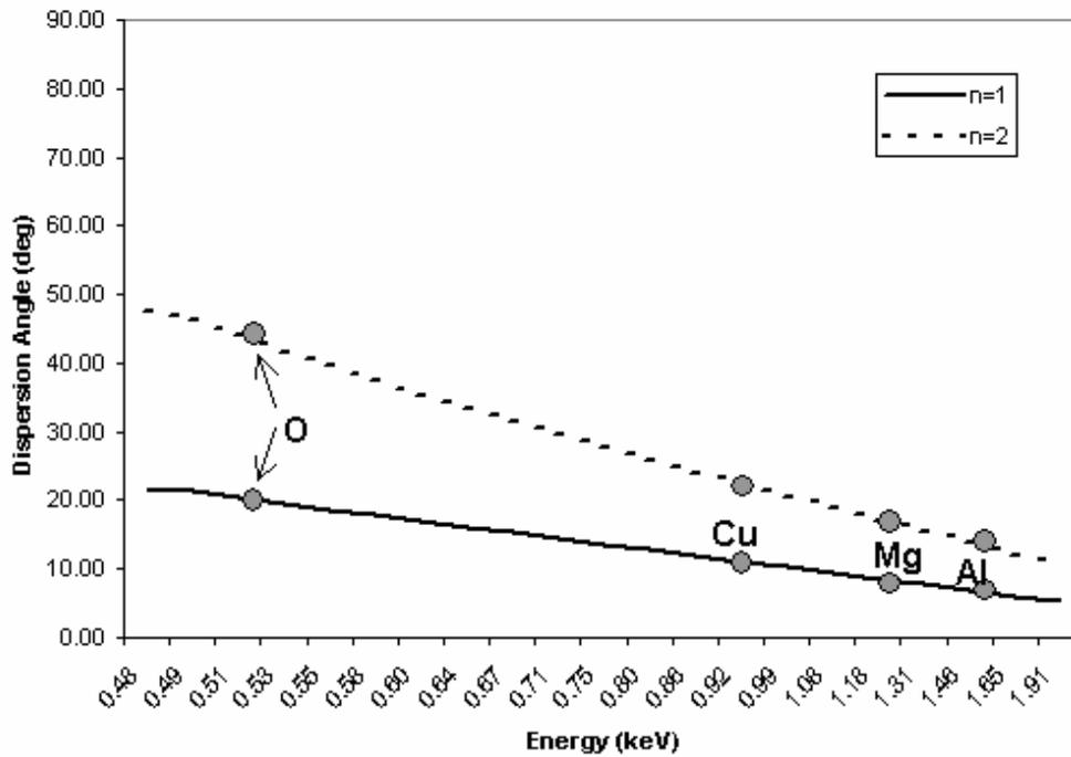
Figure 9: Predicted dispersion angles as a function of energy at first and second order. The energies of relevant lines are labeled. The graze angle on the monochromator grating is 2.0 degrees in this case.
