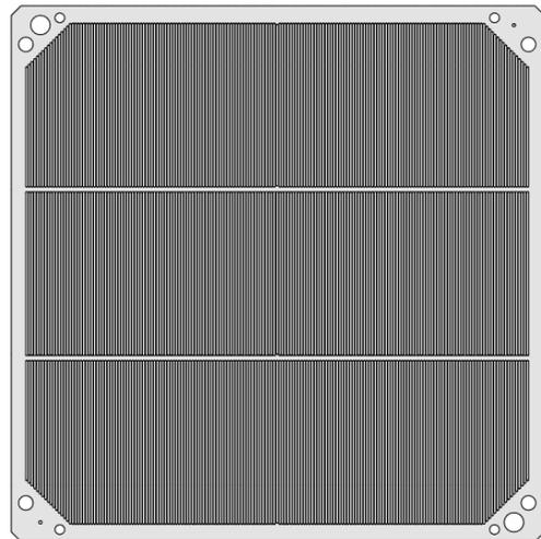
Figure 2: The top wire grid from one of the CODEX spectrometers. Each of three sections has 184 wires with 165  $\mu\text{m}$  width separated by 724  $\mu\text{m}$  gaps. The plate is 125  $\mu\text{m}$  thick electroformed nickel. The 500  $\mu\text{m}$  alignment edge is to the right, and the laser alignment holes are in the bottom right and top left.
