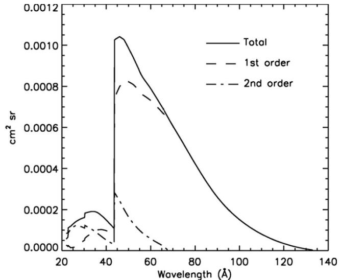
Figure 6: Effective area of the CODEX payload as a function of wavelength<sup>1</sup>.
