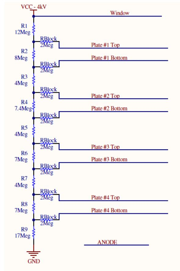
Figure 4: Electrical schematic of the CODEX GEM detectors. The 2 MΩ resistors on each plate reduce the load on other plates if one plate fails by shorting between top and bottom.
