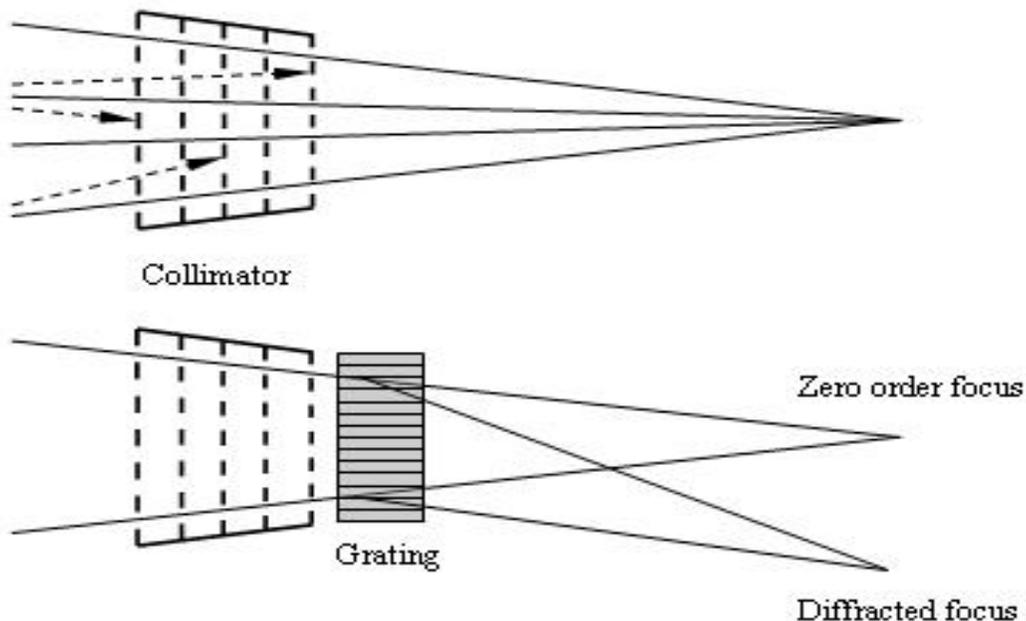
Figure 3: Schematic of the wire grid stacks ("Collimator") creating a 3.0 m focus (top) and the placement of the gratings and spectrum (bottom).
